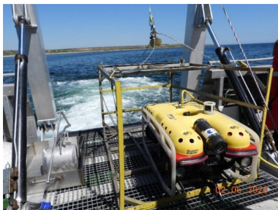
Figura IV.8 Remotely operated underwater vehicle - ROV Falcon Survey (Sursa: Blumenfield 2023)
