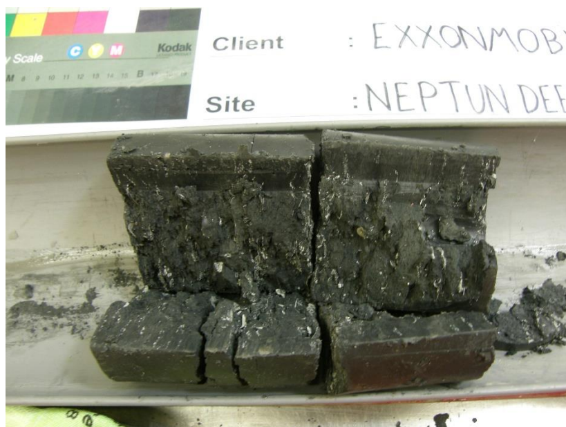
Figure 4.1: Example of shell-fragments in Geotechnical Soil Unit IV at 101.05 m PG-BH-01a
