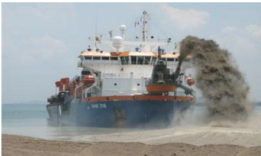
Figura 17 – Draga TSHD HAM 316 in timpul operatiunii de pompare la distanta (rainbow)
