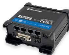
Figură 5 Router Teltonika model RUT955
